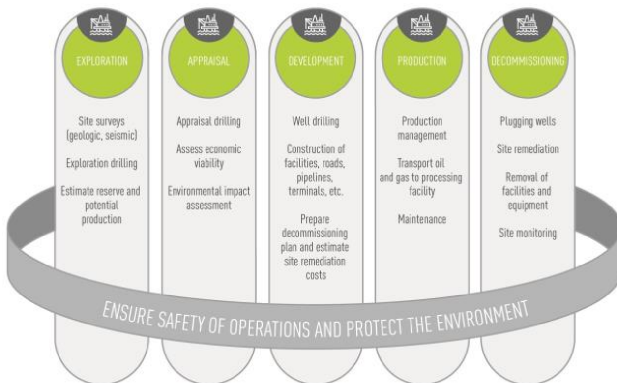
Figure 3 – Typical Life Cycle of an Oil and Gas Extraction Project (from an industry perspective)
